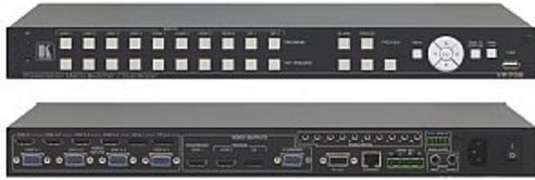
VP-732 is a 10-input presentation switcher/dual scaler with four HDMI, two DisplayPort and four user-definable (universal) analog video inputs. It up- and down-scales to selectable graphics or HDTV output resolutions to preview and program outputs (up to 4K30 UHD on the program output) and provides ultra-fast fade-thru-black switching between sources. VP-732 supports analog and embedded audio inputs and outputs and includes rich audio functionality and a stereo loudspeaker output
